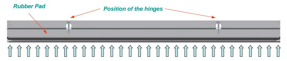
Self adjustment means constant application of load from the rubber pad to the blanket cylinder NO ADJUSTMENT REQUIRED
